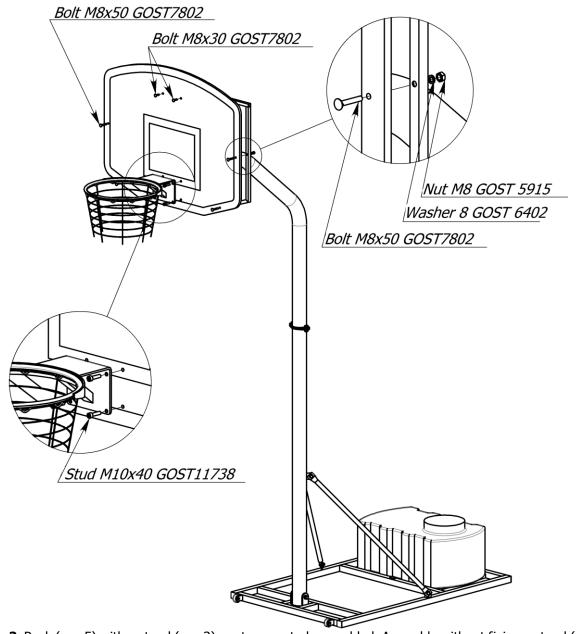
**2.** Rack (pos 5) with a stand (pos 3) are transported assembled. Assemble without fixing a stand (pos 3) with an angle beam (pos 4) in accordance with the picture below and fix the shield at the necessary height. Install a stand in a vertical position with a shield on it having assured that all the bonds are nice-fixed. Install the stand vertically with brace rods (pos 7). Metal ware is needed for fixing that is presented at the picture.
